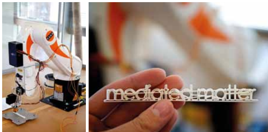
Figure 1 The multi-functional robotic arm platform configured as an ABS 3D printer (left). Printed objects have a layer height of 0.3mm (right).
