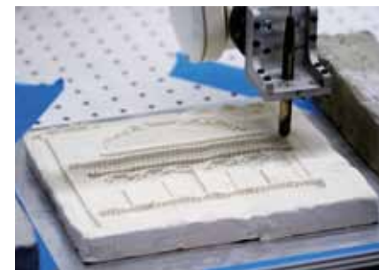
Figure 3 A clay mold is sculpted using the robotic arm platform according to a CAD file.
